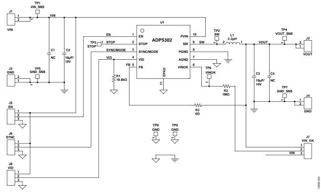
Figure 3. Schematic of the ADP5302 Evaluation Board
