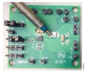
Figure 2. Output Ripple Measurement
