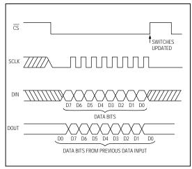
Figure 2. Three-Wire Interface Timing
