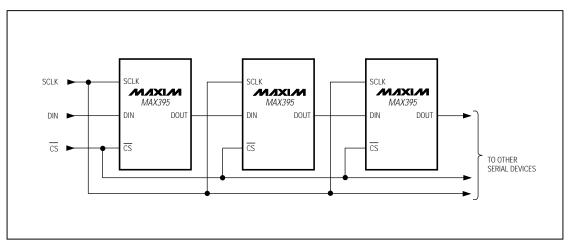
Figure 5. Daisy-Chained Connection
