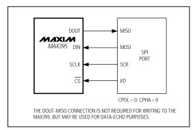
Figure 4. Connections for SPI and QSPI
