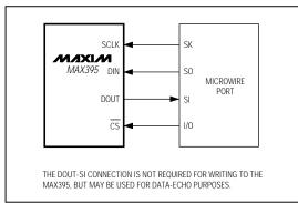
Figure 3. Connections for Microwire
