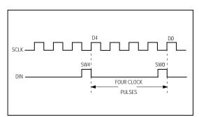
Figure 7. Differential Multiplexer Input Control
