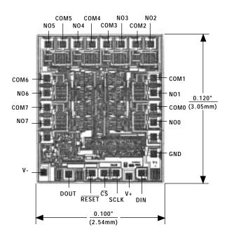
TRANSISTOR COUNT: 500 SUBSTRATE CONNECTED TO V+.
