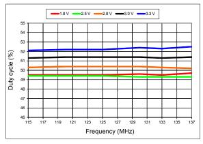
Figure 11. Duty Cycle vs Frequency
