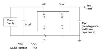
Figure 2. Test Circuit
