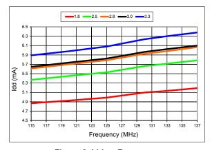
Figure 8. Idd vs Frequency
