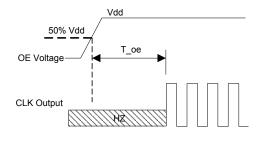
T\_oe: Time to re-enable the clock output
