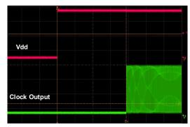
Figure 17. Startup Waveform vs. Vdd
