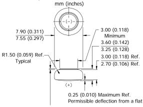
0.03 (0.001) Minimum Ref. (applies to top edge of gasket or edge of crimp, whichever is higher)
