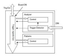
Figure 20. FPGA configuration trigger block diagram.
