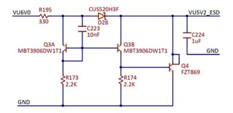
Figure Figure 7. Backpowering voltage clipper.
