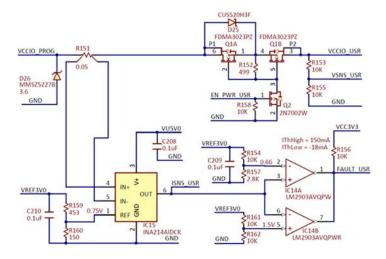
Figure 14. VCCIO\_USR protection and switch.
