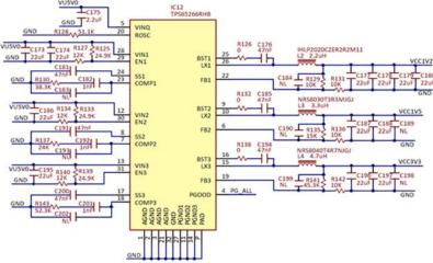
Figure 12. Internal voltage supplies.
