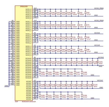
Figure 22. FPGA powering and decoupling.
