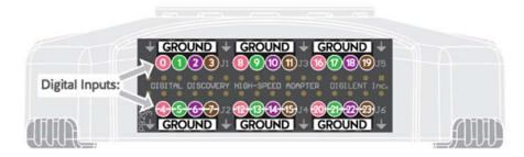
• High Speed Logic Probes (datasheet). Each twisted cable has a GND (black) wire twisted to a DIN\_USR (colored) wire. The wire connects to the High Speed Adapter via a 2 pin female header, and two 1 pin female connectors to the device under test. A 100 $\Omega$  resistor is embedded in the signal wire, on the end closest to the device under test. All GND wires should be connected to Ground of the device under test.
