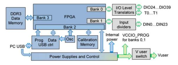
Figure 2. Digital Discovery Hardware block diagram.
