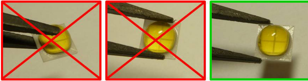
Figure 3. Incorrect handling (left and middle) and correct handling (right) of LUXEON M emitters.
