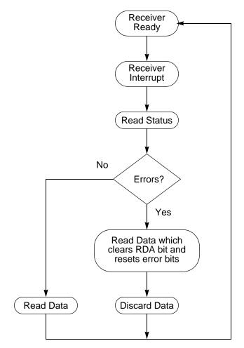
Figure 19. LIN-UART Receiver Interrupt Service Routine Flow
