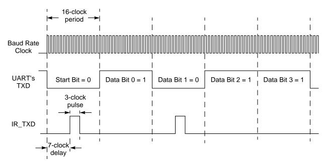
Figure 23. Infrared Data Transmission
