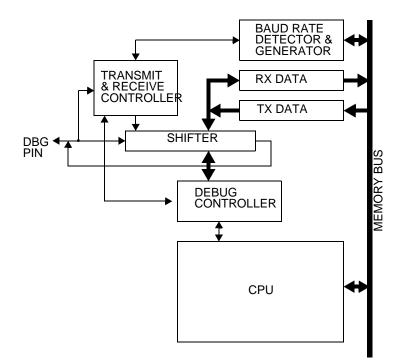
Figure 50. On-Chip Debugger Block Diagram
