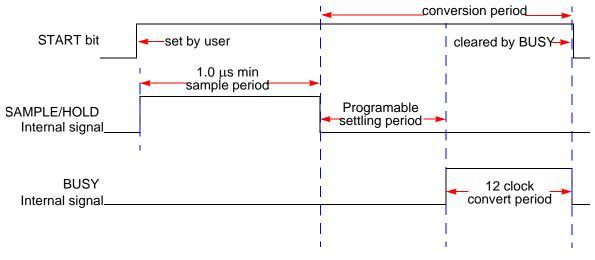
Figure 43. ADC Timing Diagram
