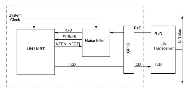
Figure 20. Noise Filter System Block Diagram
