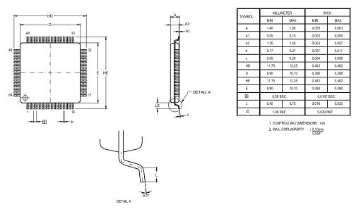
Figure 70. 64-Pin Low-Profile Quad Flat Package (LQFP)
