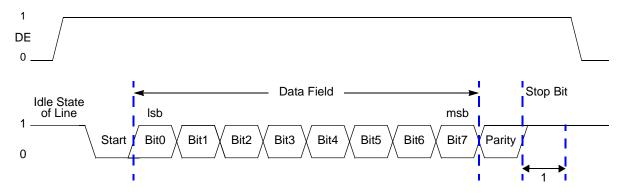
Figure 17. LIN-UART Driver Enable Signal Timing (shown with 1 Stop Bit and Parity)
