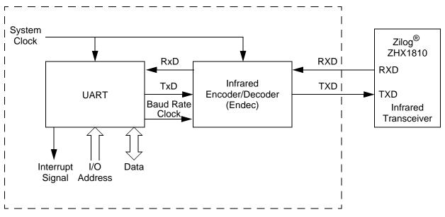
Figure 22. Infrared Data Communication System Block Diagram
