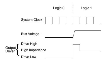
Figure 54. Output Driver when Drive High and Open Drain Enabled
