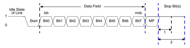
Figure 18. LIN-UART Asynchronous MULTIPROCESSOR Mode Data Format
