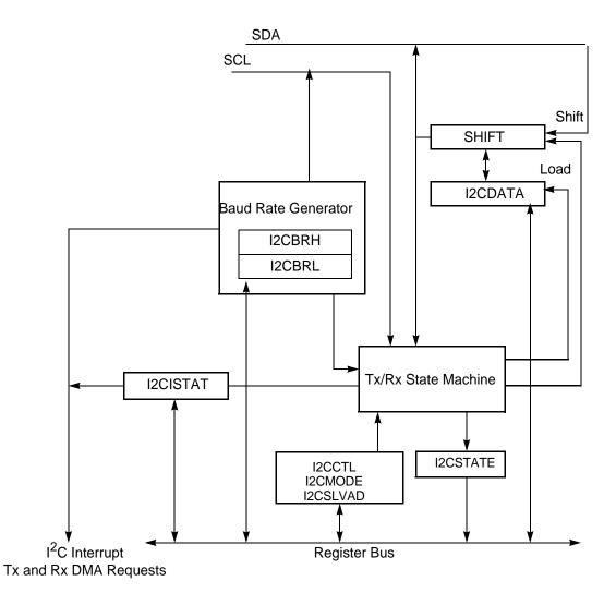
Figure 33. I<sup>2</sup>C Controller Block Diagram
