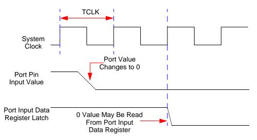
Figure 64. Port Input Sample Timing
