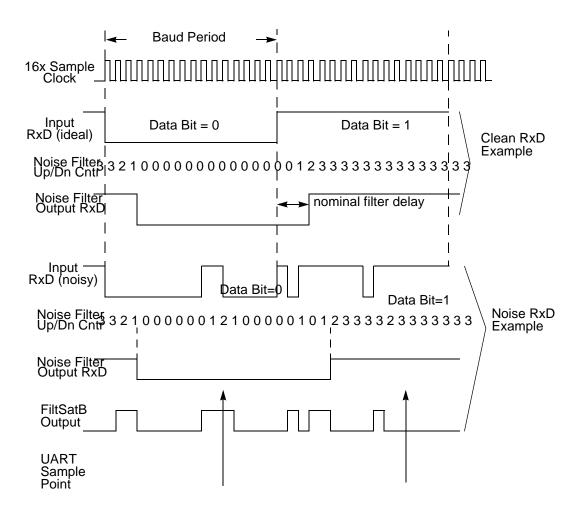
Figure 21. Noise Filter Operation
