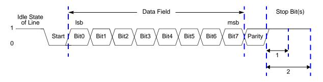
Figure 16. LIN-UART Asynchronous Data Format with Parity
