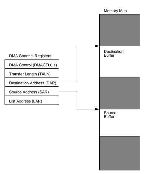
Figure 47. Direct DMA Diagram
