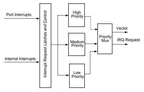
Figure 9. Interrupt Controller Block Diagram
