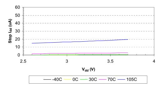
Figure 63. Stop Mode Current Versus V<sub>DD</sub>
