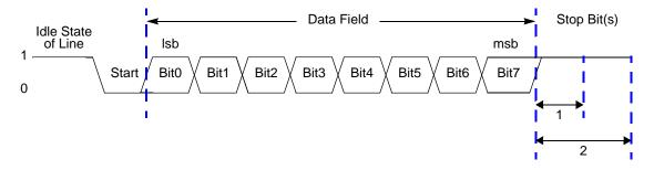
Figure 15. LIN-UART Asynchronous Data Format without Parity
