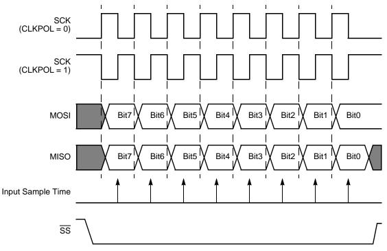
Figure 27. ESPI Timing when PHASE = 1
