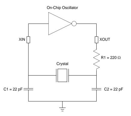
Figure 58. Recommended 20MHz Crystal Oscillator Configuration
