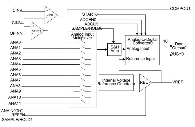
Figure 42. Analog Functions Block Diagram
