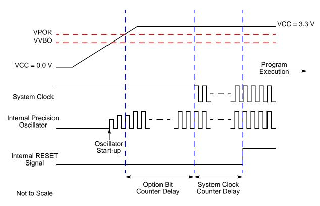
Figure 6. Power-On reset Operation
