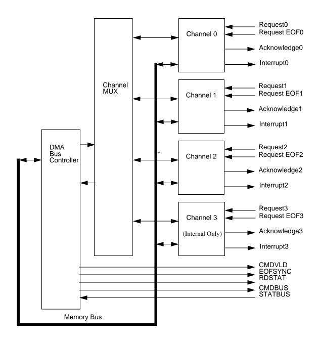
Figure 45. DMA Block Diagram
