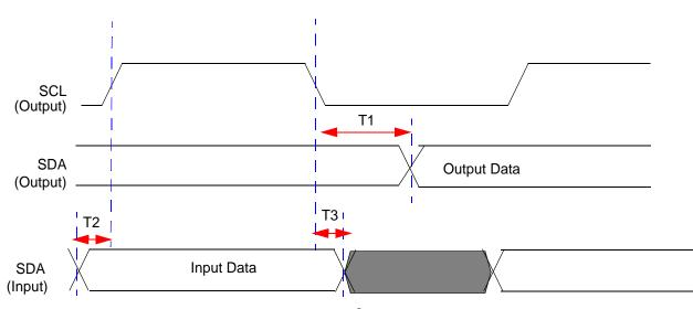
Figure 67 and Table 169 provide timing information for  $I^2C$  pins.
