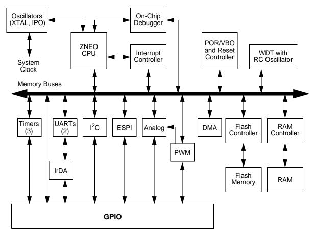
Figure 1. Z16FMC Series Block Diagram
