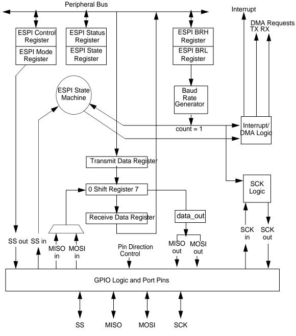
Figure 25. ESPI Block Diagram
