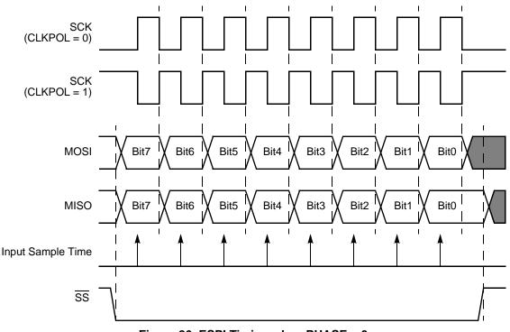
Figure 26. ESPI Timing when PHASE = 0
