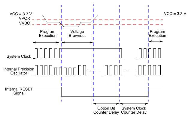
Figure 7. Voltage Brownout Reset Operation
