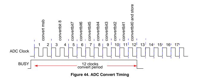
Figure 44 displays the timing of the conversion period showing the 10-bit progression of the output.
