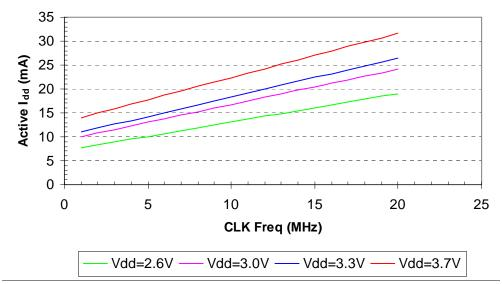
Active I<sub>dd</sub> vs CLK Freq at 30 °C
