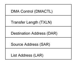
Figure 46. DMA Channel Registers
