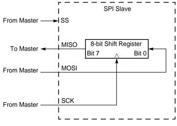
Figure 32. ESPI Configured as an SPI Slave
