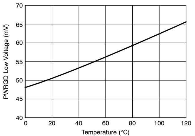
Figure 14. PWRGD Output Low Voltage vs. Temperature
