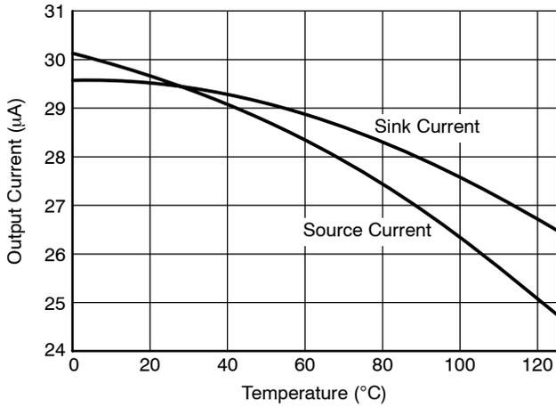
Figure 9. Error Amp Output Currents vs. Temperature
