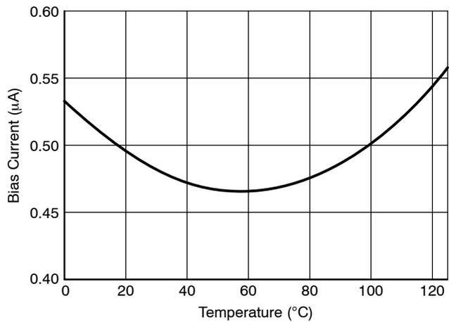
Figure 8. V<sub>FB</sub> Bias Current vs. Temperature
