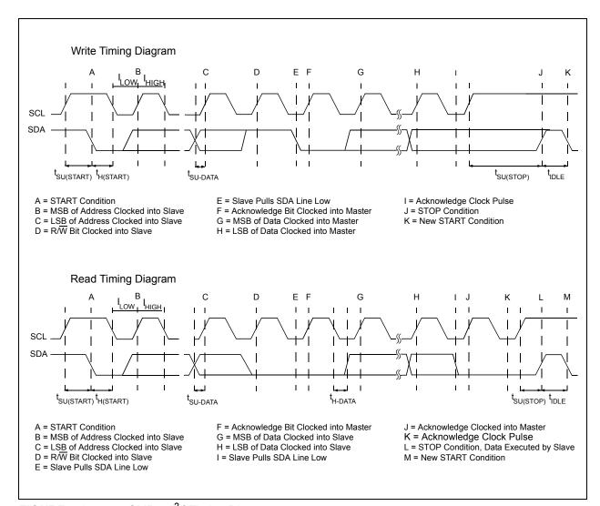
FIGURE 4-1: SMBus/I<sup>2</sup>CTiming Diagrams.
