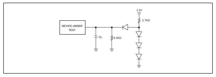
Test Condition Output Load Capacitance, CL : 1TTL gate, 30pF Rise/Fall Times : 5ns Input Pulse levels :0.0 ~ VI/O In/Out reference levels :0.5VI/O
