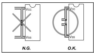
Fig. 52 Bypass capacitor across the Vss line and the Vcc line
