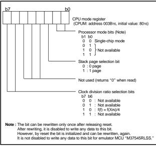
Fig. 9 Structure of CPU mode register
