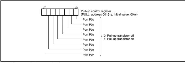
Fig. 13 Structure of pull-up control register
