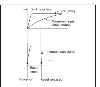
**Note:** Keep the value of supply voltage to the minimum value or more of the recommended operating conditions.
