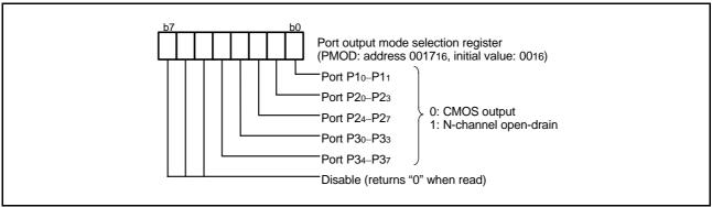
Fig. 14 Structure of port output mode selection register
