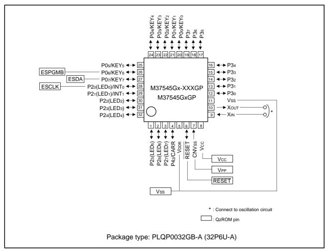
Fig. 44 Pin connection diagram (M37545Gx-XXXGP)
