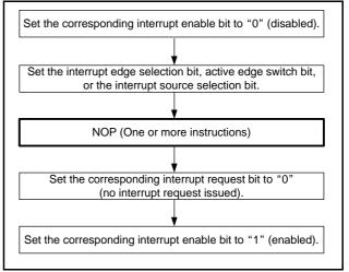
Fig 4. Sequence of changing relevant register
