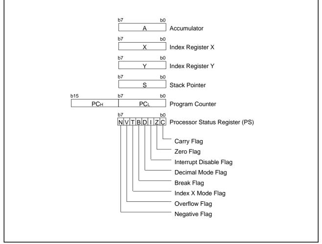
Fig. 7 740 Family CPU register structure
