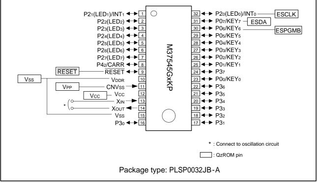
Fig. 45 Pin connection diagram (M37545GxKP)
