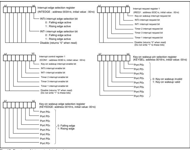
Fig. 17 Structure of interrupt-related registers
