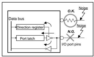
Fig. 56 Setup for I/O ports
