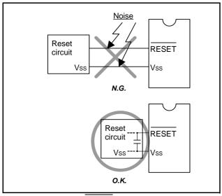
Fig. 49 Wiring for the RESET pin
