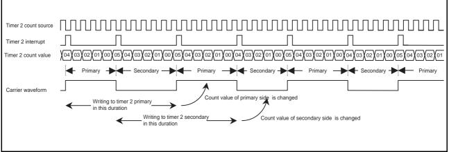
Fig. 27 Control waveform diagram of carrier wave by timer 2
