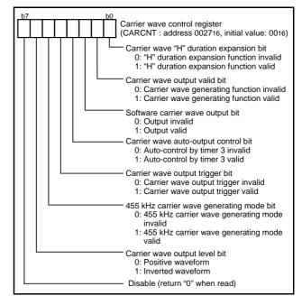
Fig. 25 Carrier wave control register
