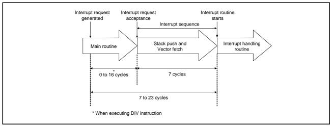
Fig. 18 Time up to execution in interrupt routine
