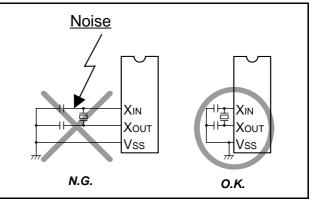
Fig. 50 Wiring for clock I/O pins
