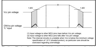
Fig 7. Timing Diagram (bold-lined periods are applicable)
