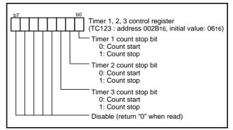
Fig. 23 Timer 1, 2, 3 control register
