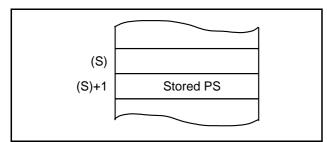
Fig 2. Stack memory contents after PHP instruction execution
