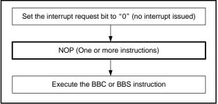
Fig 5. Sequence of check of interrupt request bit
