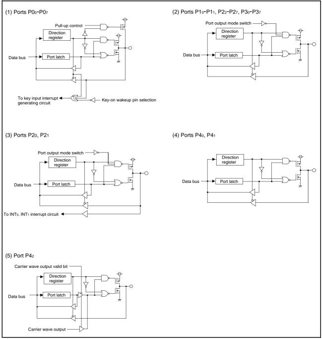
Fig. 15 Block diagram of ports (1)
