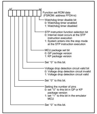
Fig. 12 Structure of Function set ROM area
