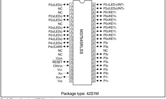
Fig. 3 Pin configuration (42S1M type)
