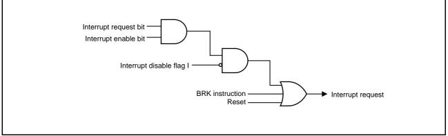
Fig. 16 Interrupt control diagram
