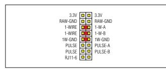
Figure 1. Jumper Settings for Parasitic Power
