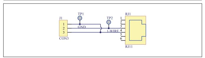
Figure 3. DS9120+ Socket Board Schematic
