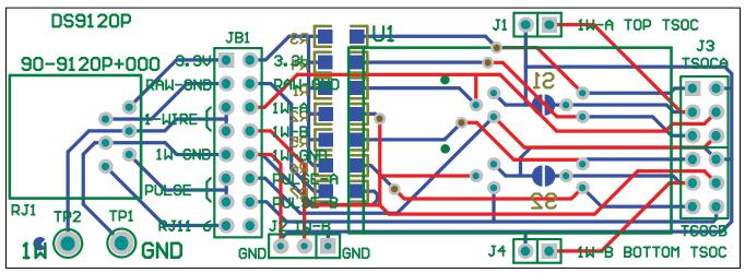
Figure 6. DS9120P+ Socket Board Composite Layout
