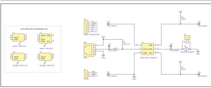
Figure 7. DS9120Q+ Socket Board Schematic
