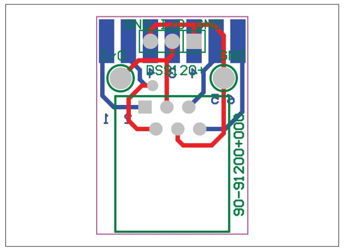
Figure 4. DS9120+ Socket Board Composite Layout
