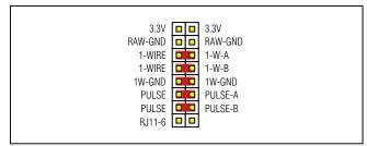
Figure 2. Jumper Settings for V<sub>CC</sub> Power and OTP Programming for DS28E10
