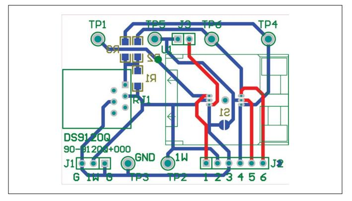
Figure 8. DS9120Q+ Socket Board Composite Layout
