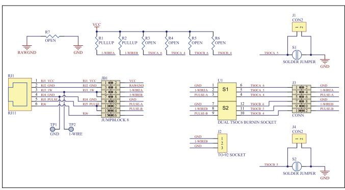
Figure 5. DS9120P+ Socket Board Schematic
