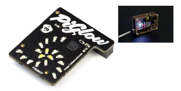
The PiGlow is a small add on board for the Raspberry Pi that provides 18 individually controllable LEDs. You can use it for all sorts of things! And of course, it fits inside a Pibow!
