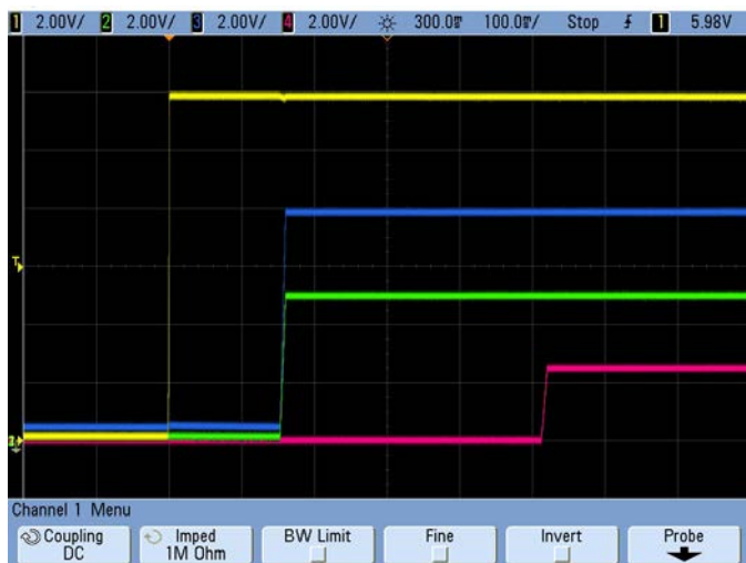
Figure 6. Sequence Timing from Board Power
