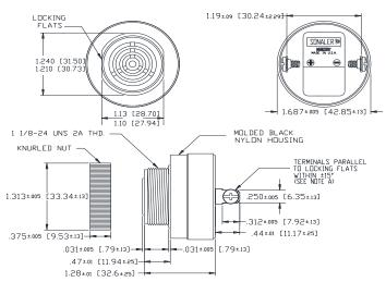
NOTE A: TERMINALS-032 BRASS TIN PLATED, TAPPED FOR #6-32 SCREW. TWO #6-32 NICKEL PLATED BRASS SCREWS INCLUBED. WILL ACCEPT 1/4' QUICK CONNECT. NOTE B. MOUNTING- REMOVE BLACK PLASTIC NUT
