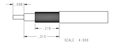
TRIMMING DIMENSIONS FOR RG-58 CABLE
