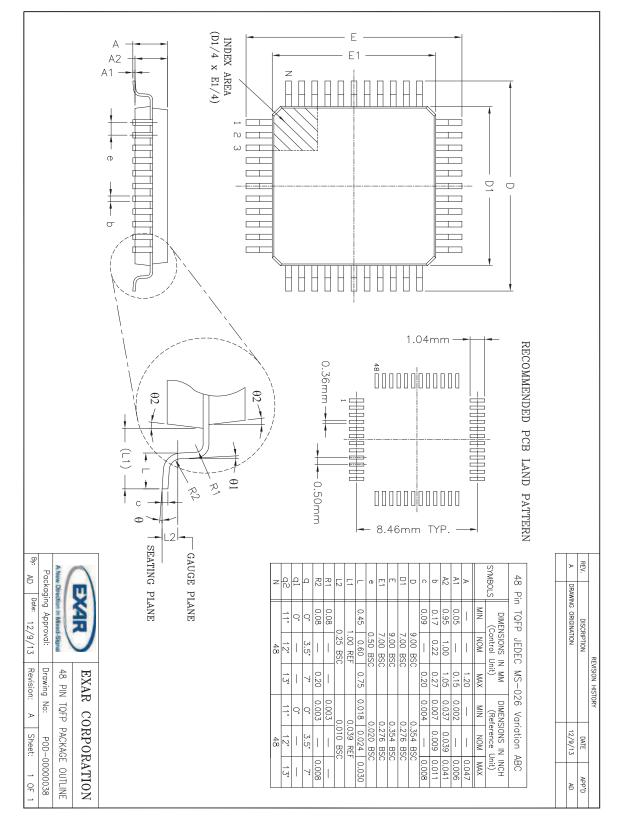
Note: TQFP48 theta ja = 64.1 deg. C/W, theta jc = 6.5 deg. C / W. All values are typical.
