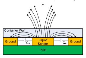
Figure 2-8. Added Capacitance (C<sub>I</sub>) When Liquid Approaches a Capacitive Sensor
