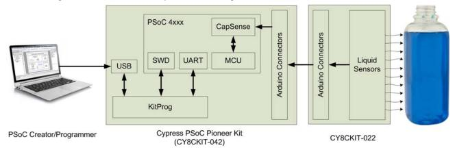
In the CY8CKIT-022 system, the CapSense circuitry in the PSoC device on the baseboard (such as CY8CKIT-042) senses the changes in the capacitance of the liquid level sensors on the CY8CKIT-022 kit. The PSoC calculates the liquid level based on the information about capacitance changes on different sensors received from the CapSense block.
