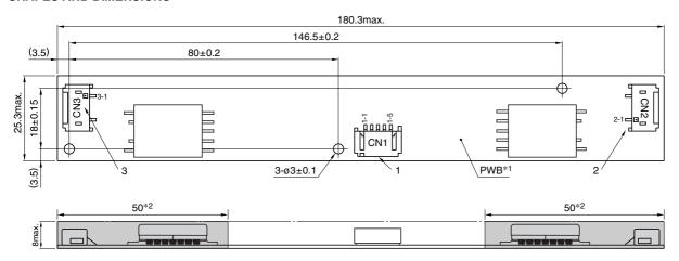
\*1 Substrate (PWB: Printed wiring board): Flame retardant UL94V-0(FR-4 or CEM-3) t=1mm
