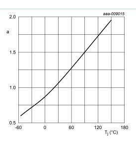
Fig. 12. Normalized drain-source on-state resistance as a function of junction temperature; typical values
