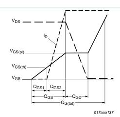
Fig. 16. MOSFET transistor: Gate charge waveform definitions
