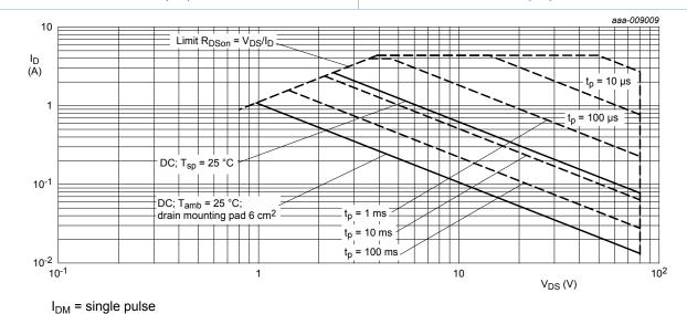
Fig. 4. Safe operating area; junction to ambient; continuous and peak drain currents as a function of drainsource voltage
