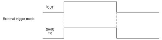
In the external trigger mode, energization is started on a rising edge of the SH/IR TR signal and stopped on the falling edge.
