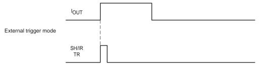
Energization starts on a rising edge of the SH/IR TR signal in the external trigger mode.
