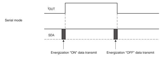
In the serial mode, energization is started by setting energization ON with serial data and stopped by setting it OFF.
