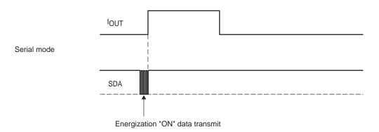
In the serial mode, energization is started by setting energization ON with serial data.
