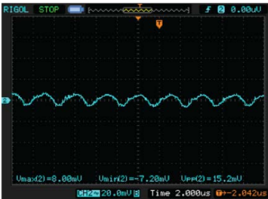
Figure 3. Output ripple at 2A load.
